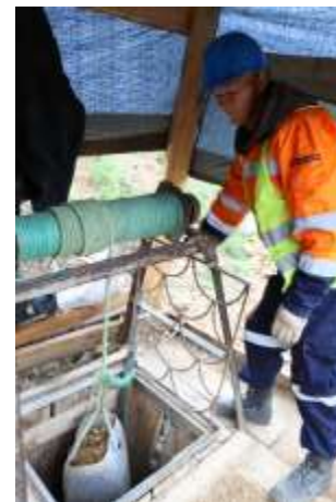
Miner operating at a secured shaft in Tunkhel village (photo taken by planetGOLD Mongolia)
