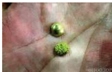
Sponge gold is the product of the gold and mercury amalgamation process (Photo taken by Today Newspaper Mongolia)
