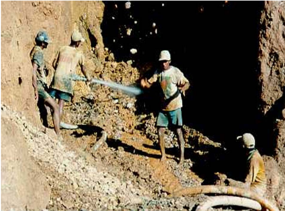
Photo 6: Hydraulic Monitoring in Brazil – Undercutting of Hill Slopes is a Frequent Occurrence (Photo by J. Hinton)
