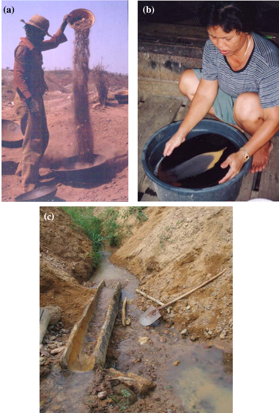
Photo 4: Gravity Separation by (a) Wind Sorting, (b) Panning and (c) Simple Log Sluice (Photos by (a) H. Wotruba; (b) M. Veiga and (c) R. Gaucher)
