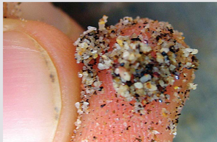
Tiny mercury droplets can be seen in the feed material at operations that practice whole ore amalgamation before cyanidation.
