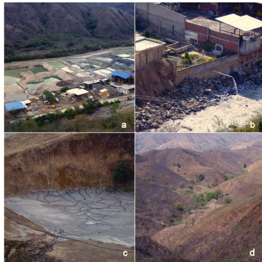
Poorly managed waste, contaminated sites, and a solution for artisanal and small scale gold mining in Portovelo, Ecuador: (a) substandard tailings ponds; (b) direct discharge to rivers; (c) site contaminated with tailings; (d) solution: an adjacent valley (burned pasture) that is a suitable for a tailings impoundment that meets international standards and that can serve the needs of the ASGM community.
