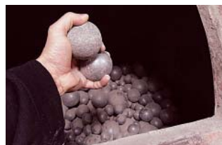
Rocks are crushed manually using hammers, and then milled using ball mills (Tanzania, 2010).
