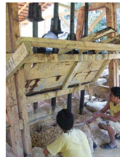
Stamp mill for reducing rocks to pea-sized particles (Sulawesi, Indonesia, 2007).
