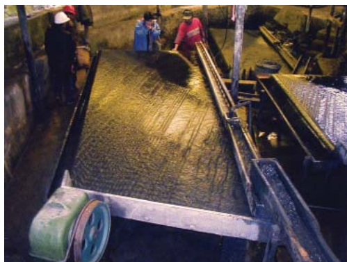
A large shaking table in operation (Mongolia, 2010).
