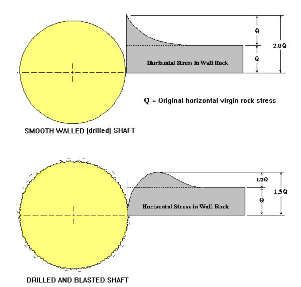
Figure 2-1 Induced Stresses around Shafts
