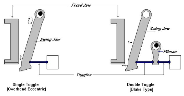
Figure 25-1 Jaw Crusher Types
