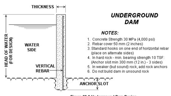
Figure 20-3 Underground Dam Design
