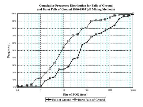
Figure 2-5 Falls of Ground Compared to Rockbursts
