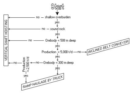
Figure 4-1 Moving Ore to Surface
